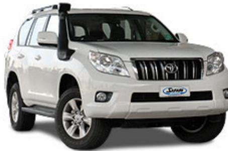
Pioneered in Australia in the early 1980's, Safari Snorkels were born out of a need to protect 4WD engines from the hazards of dust and water commonly encountered in touring and off road applications.
