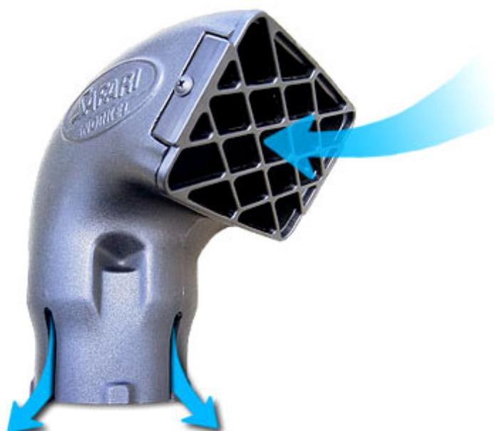
altitude conditions where heavy snow falls are anticipated. By rotating the air ram to face away from the prevailing wind/direction of motion, the air ram delivers additional protection from the choking effects of snow build-up inside the air intake.
