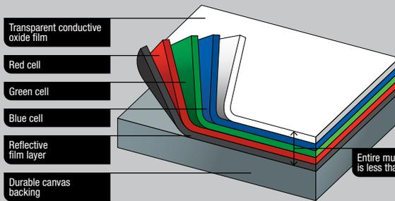
Redarc amorphous solar blankets utilise unique triple-junction amorphous silicon solar cells, where the blue, green and red light spectrum of the sun is absorbed in different layers of the cell.
